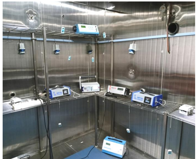
^{222}\text{Rn} Chamber at CARER, Mangalore University
